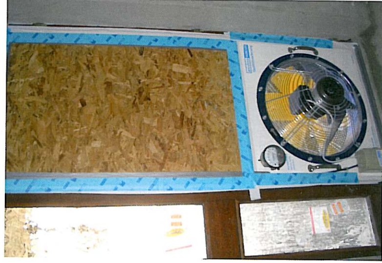
The Wincon test in progress on one of the units at Castlemagner.
